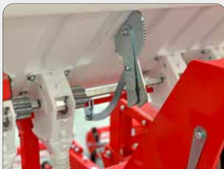
Lid system discharge all fertilizer in the ho
