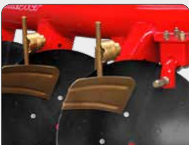
Mud Scraper Adjustable mud scrapers are placed in the machines so as to prevent accumulation of the mud.
