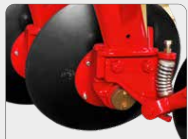
Position Angle Disc has two positions, one of them is direction angle and the other one is position angle. Position angle is adjusted from the slots on disc brackets.
